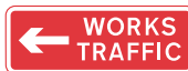
Sign to direct works traffic in advance of a road junction or works entrance
