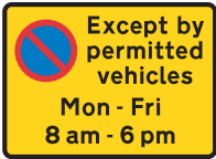
Repeater sign within a loading area
