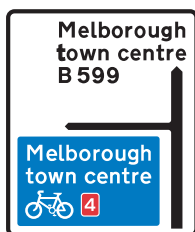
Non-primary route direction sign, in advance of a junction, indicating a route for cyclists
