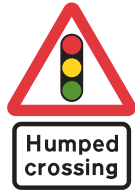
Signal-controlled pedestrian crossing on a road hump
