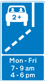
Start of HOV lane (near-side)
