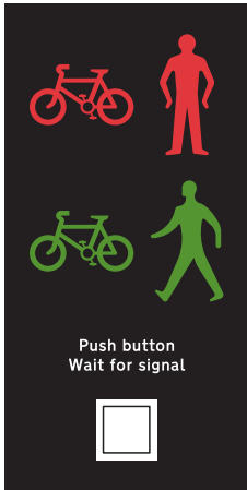
Near-side signals for Toucan crossing
