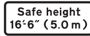
Electrified overhead cable and the safe height beneath it (usually associated with an overhead electrified railway or tramway). On the approach to a junction, the plate may include an arrow to indicate the direction of the level crossing
