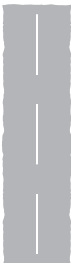
Hazard warning line (replaces a centre line or a lane line). An upright sign may indicate the nature of the hazard, such as a bend. The marking is used also on the approach to a junction
