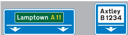
Appropriate lanes to use on the approach to the junction (overhead sign over the slip road)
