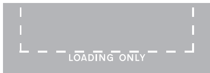
Loading bay (conditions of use shown on upright sign)
