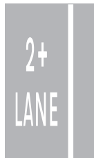
HOV lane road marking
