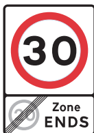
End of 20 mph zone and start of 30 mph speed limit
